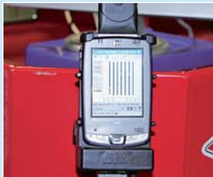
Soil Essentials’ ‘CropCircle’ sensor, which scans and measures the leaf area index of a crop, can vary fertiliser applications in ‘real time’. The sensor and control box adjust the rate, on the move, relative to recommendations in the HGCA wheat growth guide.
